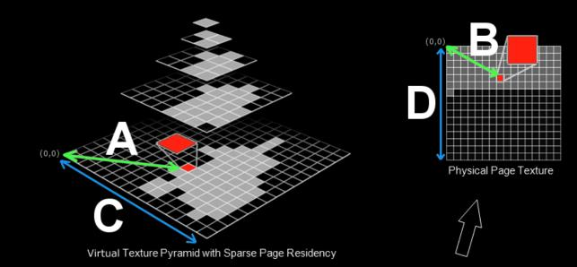
scale = C / D bias = B - A × scale physical = virtual × scale + bias
